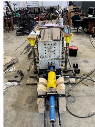
Figure 3c. Prestressing bed setup and distributed strand setup for reading strain from BOTDR.
