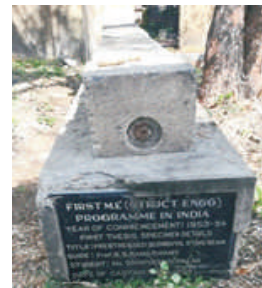
The first M.E. (Structural Engineering) thesis specimen on prestressed segmental stone beam in the year 1954, preserved at Annamalai University, Chidambaram, Tamil Nadu (Photo Courtesy: Er M. Durai)
