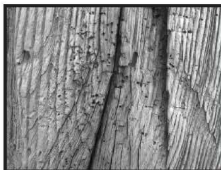
Fig. 1. Damage To Wood Caused By The Sun
