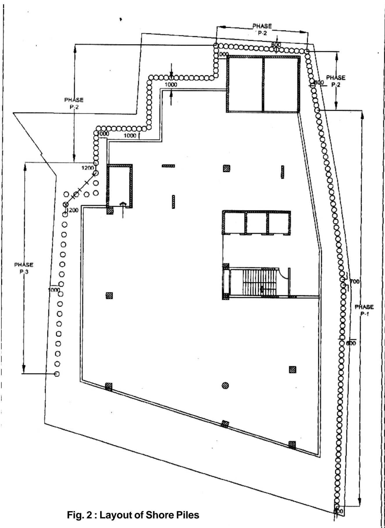
**Fig. 2 : Layout of Shore Piles**
