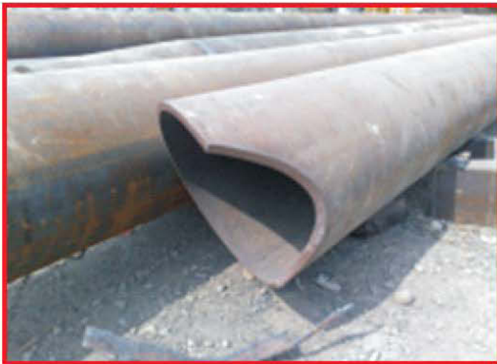
Fig.13: CHS Profile Cutting
