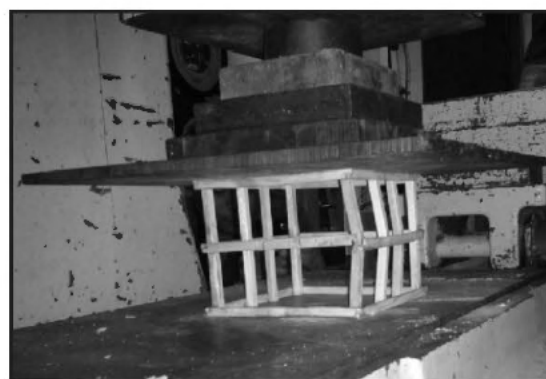
Figure 4. Compression test of prototype (buckling of columns at middle beam joints observed)
