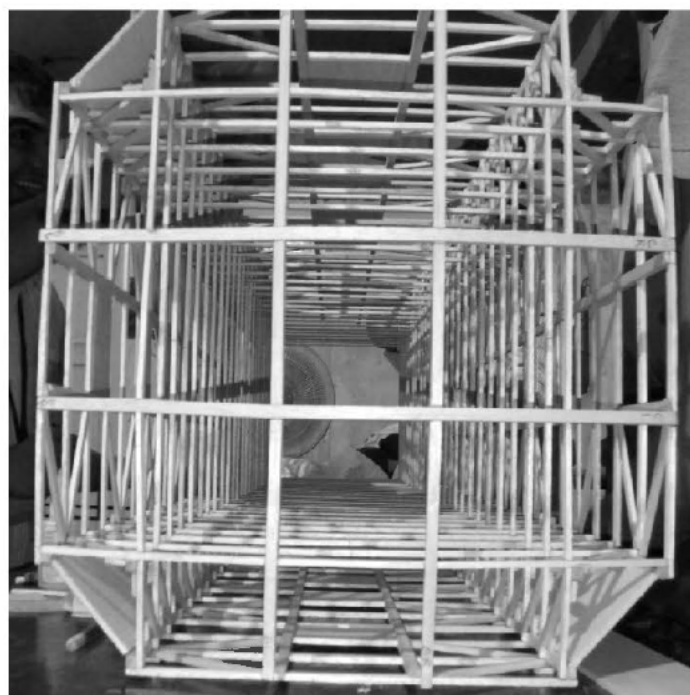
Figure 6: Thicker members in Roof grid
